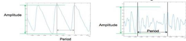
Figure 1. Example of PPG and BCG waves, respectively
